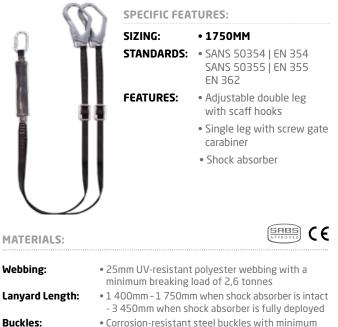
• Corrosion-resistant steel buckles with minimum breaking force of 18kN • Corrosion-resistant steel scaffolding hooks: 50mm
